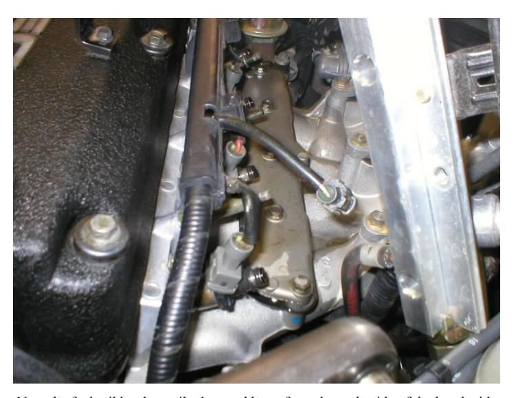
Now the fuel rail has been tilted up and hung from the underside of the hood with the bungee cord, the EGR runner housing is at last in sight. Remove the 10mm bolts that hold it to the intake manifold, when it is loose grab it and the gasket and take them off the manifold
