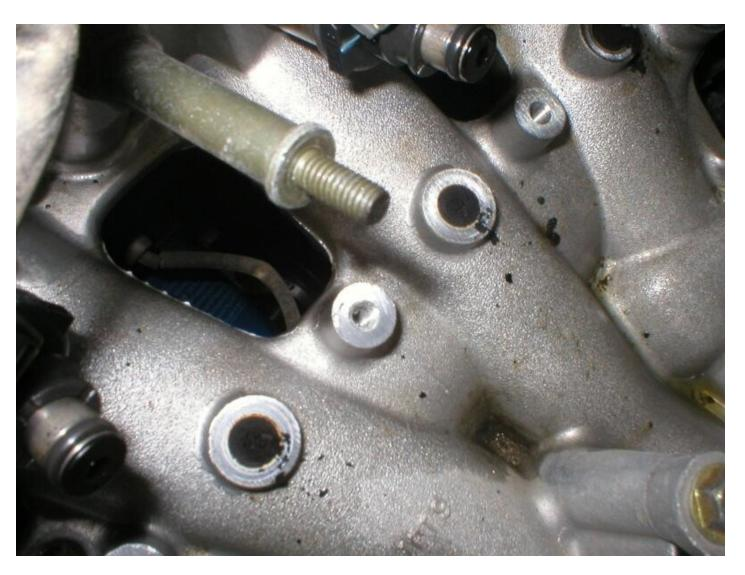
The ports in the intake are plugged up, use the drill bit and start 'hand' drilling into the ports to remove the blockage, keep blowing the dust away. When the drill bit goes all the way thru you can use the side of the drill bit to "rod out" the rest of the hole. the ports are of different sizes and you don't want to expand the hole size with the drill bit, just get all the carbon out.
