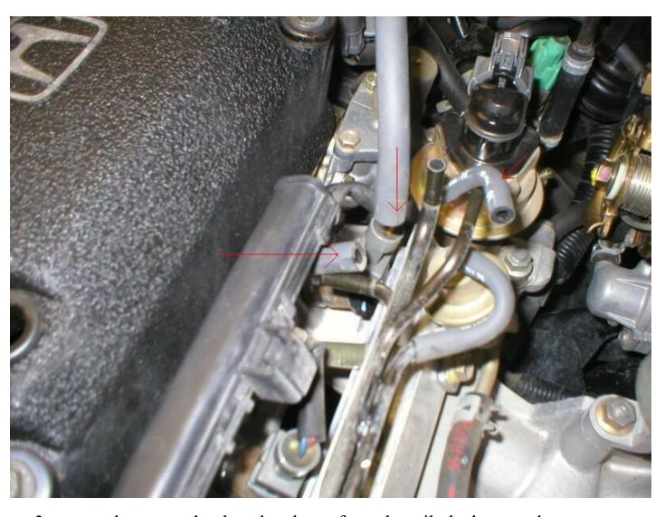
3 vacuum hoses need to be taken loose from the rail, the hose to the pressure regulator can stay hooked up
