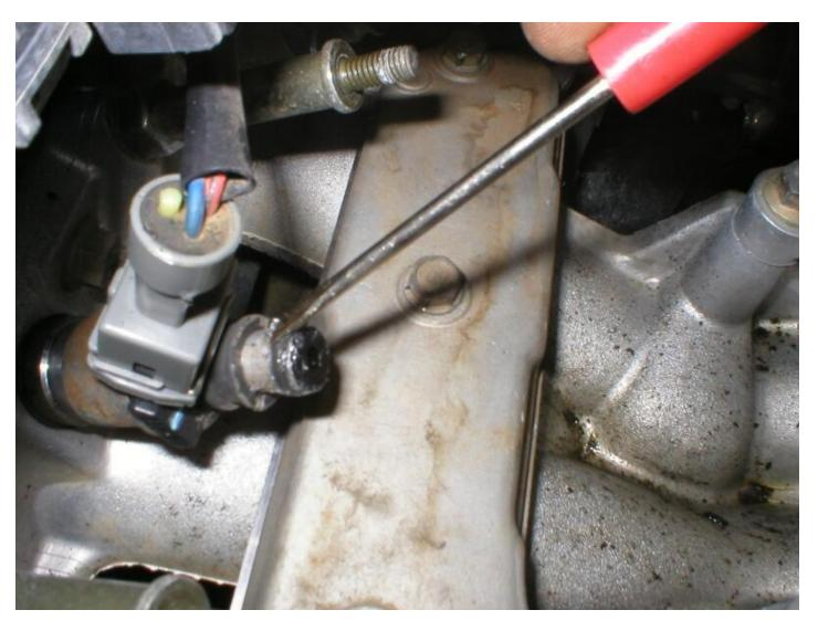
Reassemble everything in reverse order when it is all cleaned. All the 10mm nuts&bolts are around 10ftlbs torque. Before you put the fuel rail back on it's a good idea to put a light smear of silicone grease on to the injector 'O'rings to help them seat. Check for leaks after the engine is restarted.
