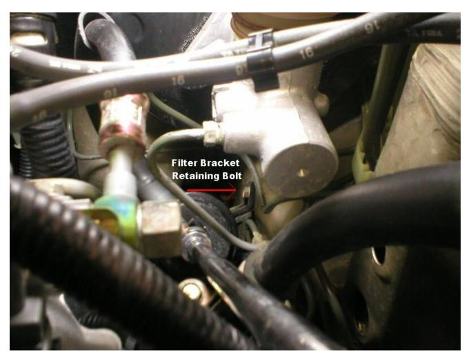
Now the bracket and filter are held on by one 10mm bolt, the lower part of the bracket is a tab/slot setup.
