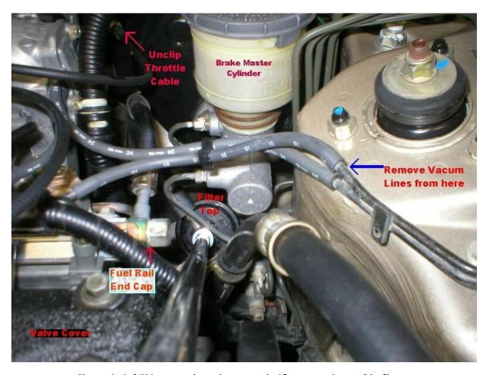
Here again the 3/8" impact can be used to remove the 17mm nut on the top of the filter.
