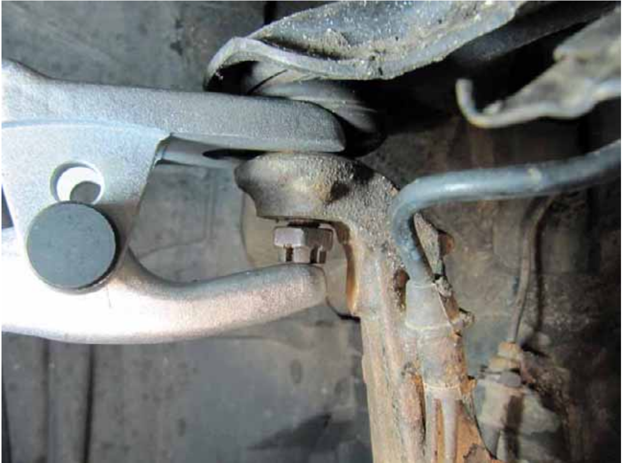
#16 – Side view showing placement of the ball joint separator.
