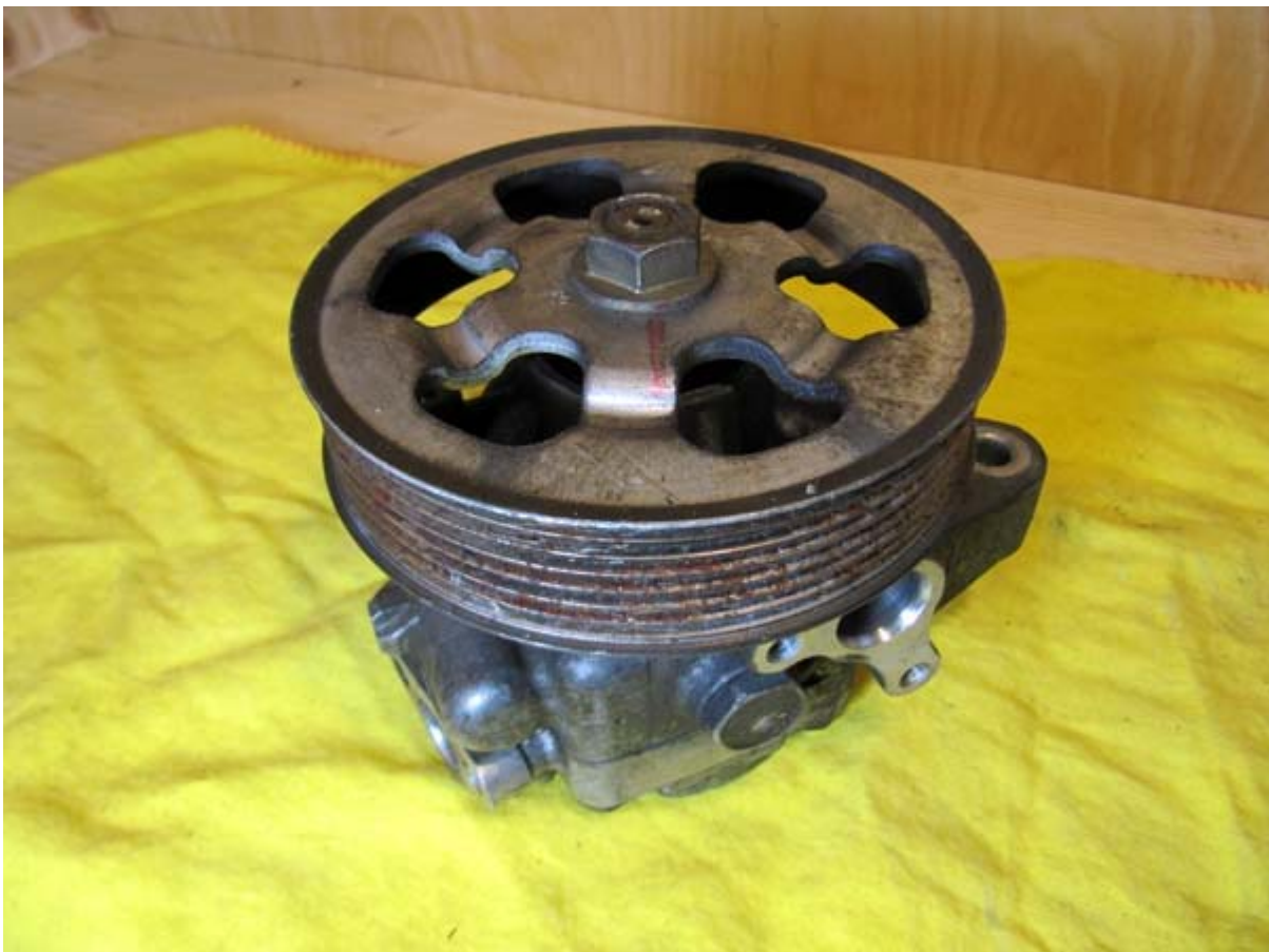
Honda 2007 4CYL Power Steering Pump
