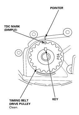
Set the camshaft pulley so that the No. 1 piston is at TDC.
