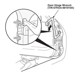
3. Check the door gaps on the top, bottom, and sides. The top and bottom gaps should be equal, and the side gaps should be equal.
