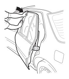
9. Inspect the fit of the weatherstrip between the back of the rear door and the C pillar. The weatherstrip should just touch the C pillar, or there should be a small air gap. If the fit is too tight and the weatherstrip folds over as the door is opened, shift the weatherstrip forward and outward.
