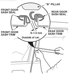
8. The rear door sash should also be recessed slightly behind the front door sash. If the rear door seal overlaps the front door seal, or the rear door sash is not recessed, bend in the top of the rear window frame. Place a rubber mallet between the rear door and the body. Close the door against the mallet; then push on the top front corner of the rear door window frame to bend it in.
