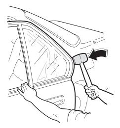
Reinspect the fit of the weatherstrip along the C pillar.
