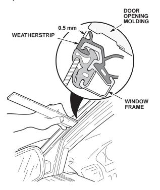
To adjust the window frame, lower the window. Place a mallet head or block of wood between the window frame and the body at the A pillar. Close the door against the mallet or block and carefully push on the door to force the window frame outward.
