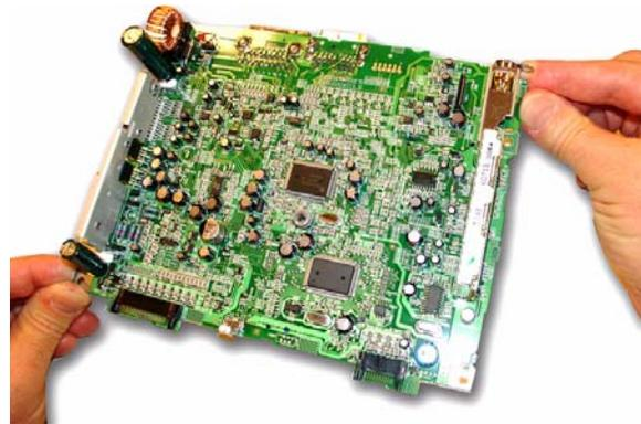
11. Set the PCB next to the audio unit on the ESD mat, and pull on the ribbon cable to disconnect it from the PCB.
