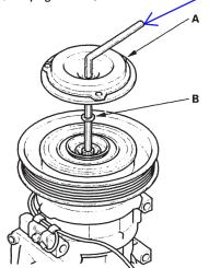
If you are replacing the field coil, remove the snap ring (A) with snap ring pliers, then remove the pulley (B). Be careful not to damage the pulley and compressor.
