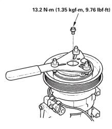
2. Remove the pressure plate (A) and shim(s) (B), taking care not to lose the shim(s). If the clutch needs adjustment, increase or decrease the number and thickness of shims as nesessary, then reinstall the pressure plate, and recheck its clearance (see page 21-50).
