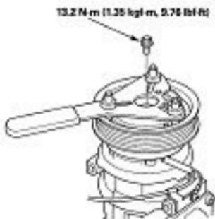
2. Remove the pressure plate (A) and shim(s) (B), taking care not to lose the shim(s). If the clutch needs adjustment, increase or decrease the number and thickness of shims as necessary, then reinstall the pressure plate, and recheck its clearance (see page 21-20).
