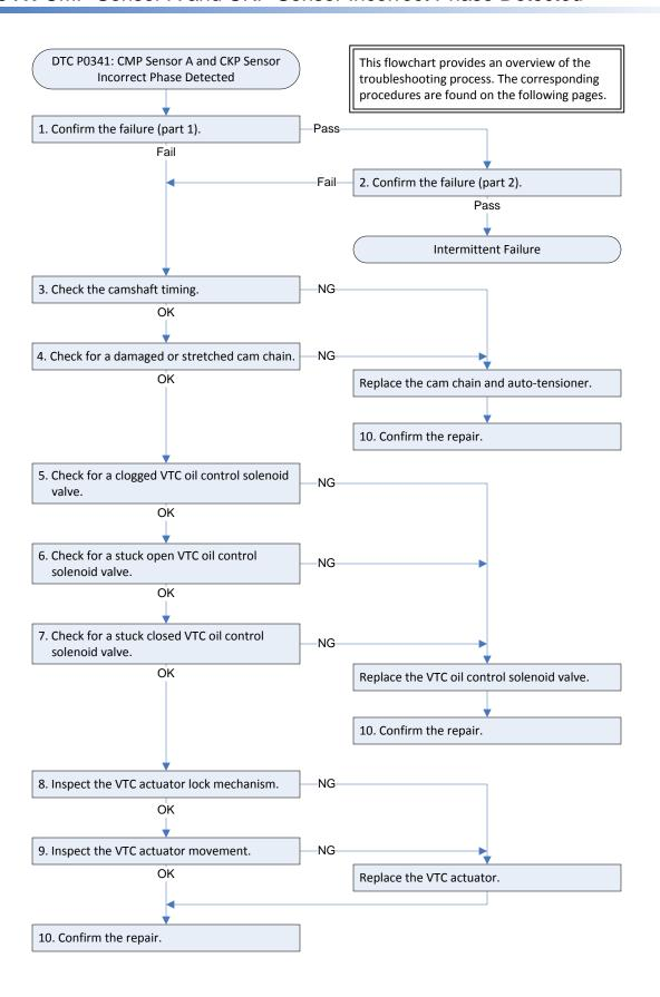
**DTC P0341:** CMP Sensor A and CKP Sensor Incorrect Phase Detected
