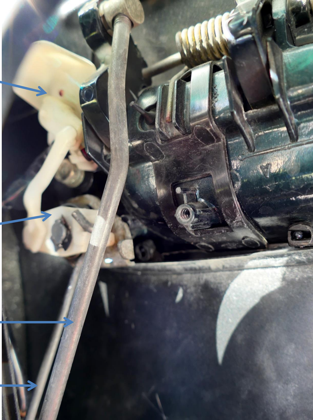
Photo of Middle Inside Left Front Door of 1994 Accord Showing Key- Driven and Handle-Driven Mechanical Lock and Latch Actuator Assemblies
