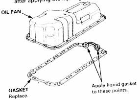
20. Tighten the nuts finger-tight at six points as shown
