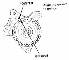
17. Check alignment of pointers after installing the gear
