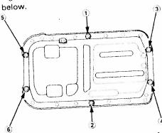
21. Tighten all bolts and nuts, starting from nut (1)clockwise in three steps.
