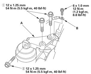
6. Install the ground cable (B).
