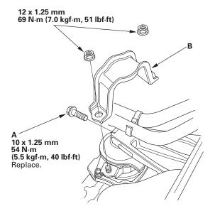
5. Install the upper bracket (A), then tighten the bolts in the sequence shown.
