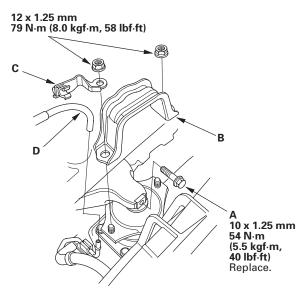
4. Tighten the rear mount bolt (A), then install the rear mount stop (B).
