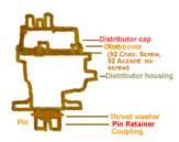
**Top:** How to remove the covers and various parts from the distributor housings is shown above in gif animation. **CAUTION:** Do not tap on the rotor to remove it, instead use large flat head screw drivers. If the rotor doesn't come off then crush it with a vise grip. Do not work with the ignition system with the ignition ON.
