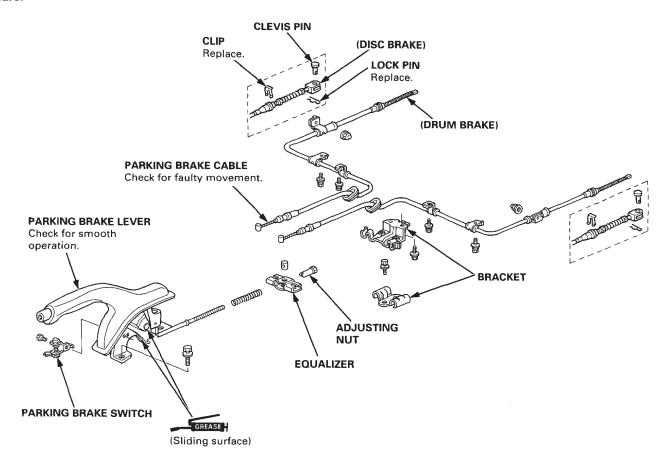
Disconnect the parking brake cable from the lever on the caliper by removing the lock pin and clevis pin, and remove the cable from the arm by removing the clip.
