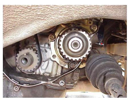
As you look at the sprocket on the right, this sprocket is connected to another gear on the inside of the gear case that meshes with the gear on the end of the rear balance shaft. This sprocket is an integral part of the Rear Balance Shaft Gear Case.
