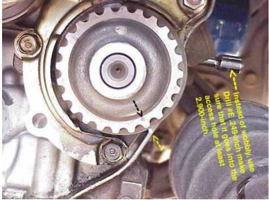
There is a service cap plug that unscrews in the side of the block (Image Below), remove it and insert a 4 inch wobbly 1/4 inch drive extension the wobbly end in first (USE THE DRILL IF YOU CAN FIND ONE CHECK WITH ACE HARDWARE OR AN AUTOMOTIVE STORE... THEY CAN ORDER ONE FOR YOU).
