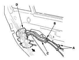
Remove the maintenance hole seal (A) and bolts, slide the protector (B) ('03 model) or the outer handle bracket (C) ('04-06 models) rearward, then remove it.
