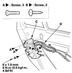
4. Detach the cable clips (A) and the hook (B) of the cable protector (C), then pull the latch (D) and the cable protector forward. Take care not to bend any of the cables.
