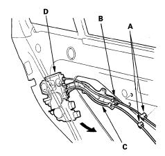
7. Remove the cable protector (A) from the latch protector (B) by releasing the hook (C).
