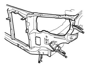
Measure the front compartment diagonally.
