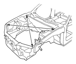
9. Temporarily assemble the hood, headlight and front fender, then check the clearances and level differences.
