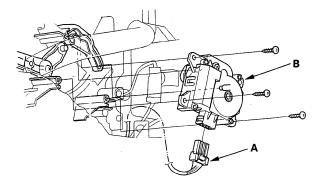
3. Install the motor in the reverse order of removal. After installation, make sure the motor runs smoothly.
