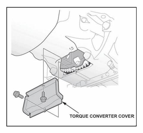
12. Remove the torque converter cover.
