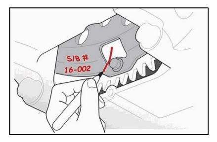
15. Mark the torque converter and the flex plate as shown. Then, write the bulletin number (16-002) on the flex plate with a permanent marker or paint marker.
