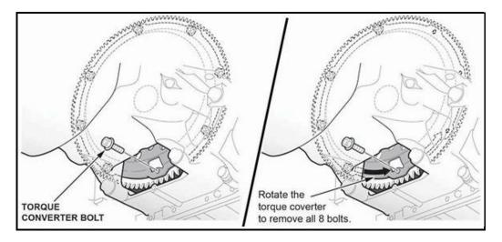
13. Rotate the crankshaft and remove all eight bolts.
